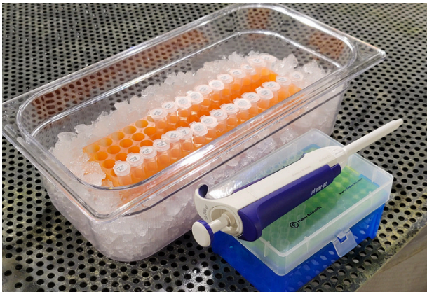
Figure 4: 20µl-200 µl micropipette for milt collection from male lake whitefish ( C. clupeiiformis ).
